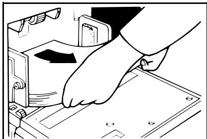
**2** Adjust the paper feed side plates to match the paper size.
