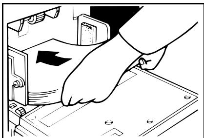
**4** Make sure that the paper feed side plates contact the paper lightly.
